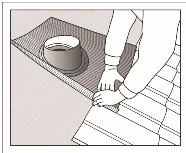
**Figure 7 Interlocking tile flashing installation**
