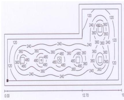
Dialux plot showing the average Lux levels delivered from 6 Solatube® 330 DS-C Tubular Daylighting Systems at the E.ON office.
